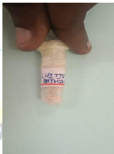
Fig 3: Extracted Chitin from Shrimp shells
